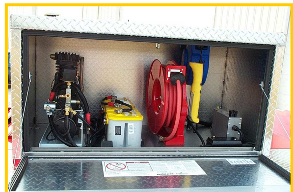
Street side mounted accessory compartment with air compressor, air hose reel, LED trouble-light reel and 110V GFI outlet.
