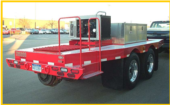
Heavy duty, compact towing package with stylish aluminum deck plate coverings, full width bumper with LED lighting, and integral steps.
