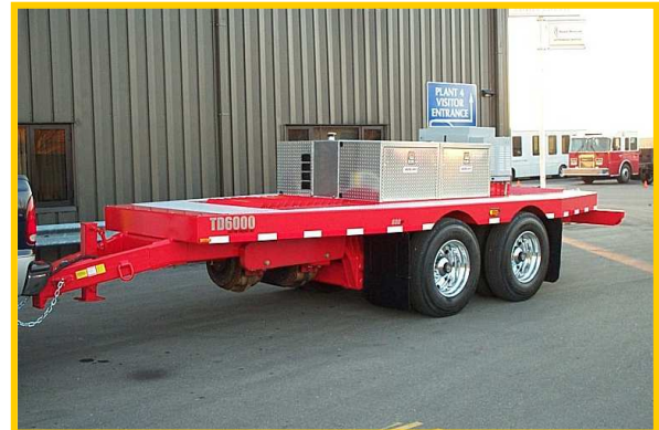
8' x 3' x 1/4" thk tubular frame with integral drop tongue and 30,000 lb adjustable pintle hitch.
