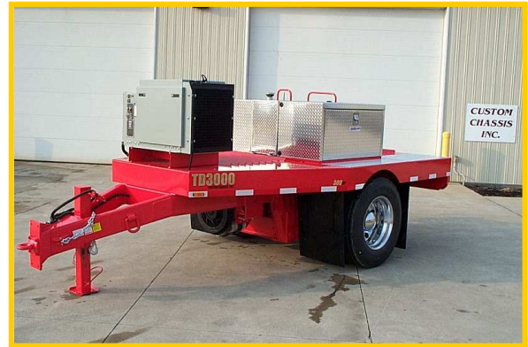
8" x 3" x 1/4" thk tubular frame with integral drop tongue and 30,000 lb adjustable pintle hitch.
