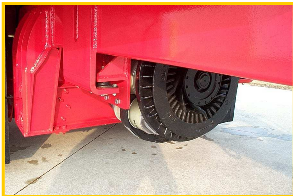
Rubber mounted PAUs for reduced frame stress.
